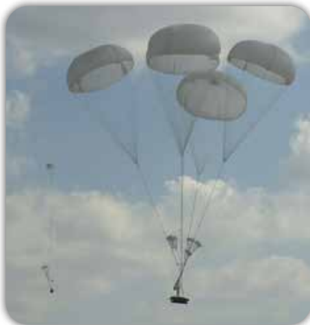
Platform Sub-system with Payload in Air with Deployed Parachute Sub-system
