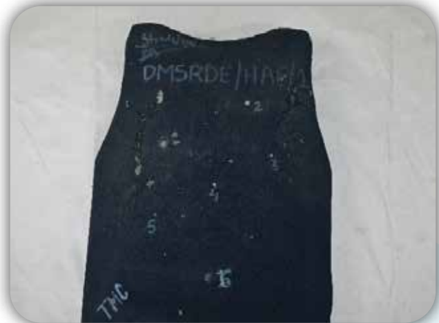
Tested Hard Armour Panels (HAPs) against multiple hits of 7.62x54mm R API
