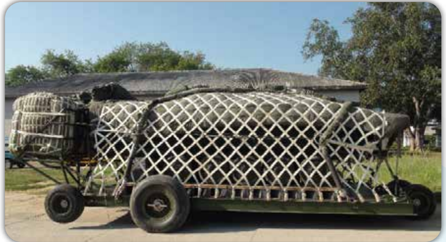
Platform Sub-system with Payload & Parachute Sub-system in Packed Condition
