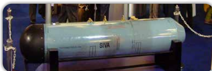
Pod Shell with Rocket Pod Adapter
